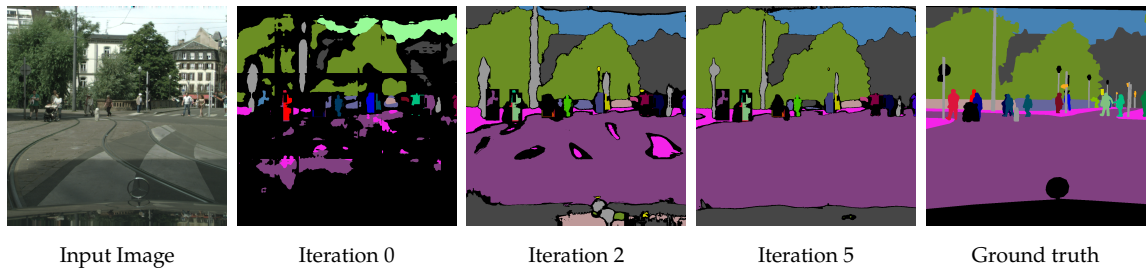
Figure 5.4: By using the output of the trained network, the initial approximate ground truth produced according to Sec. 5.3.2 and 5.3.3 (Iteration 0) can be improved. Black regions are “ignore” labels over which the loss is not computed in training. Note for instance segmentation, permutations of instance labels of the same class are equivalent.
