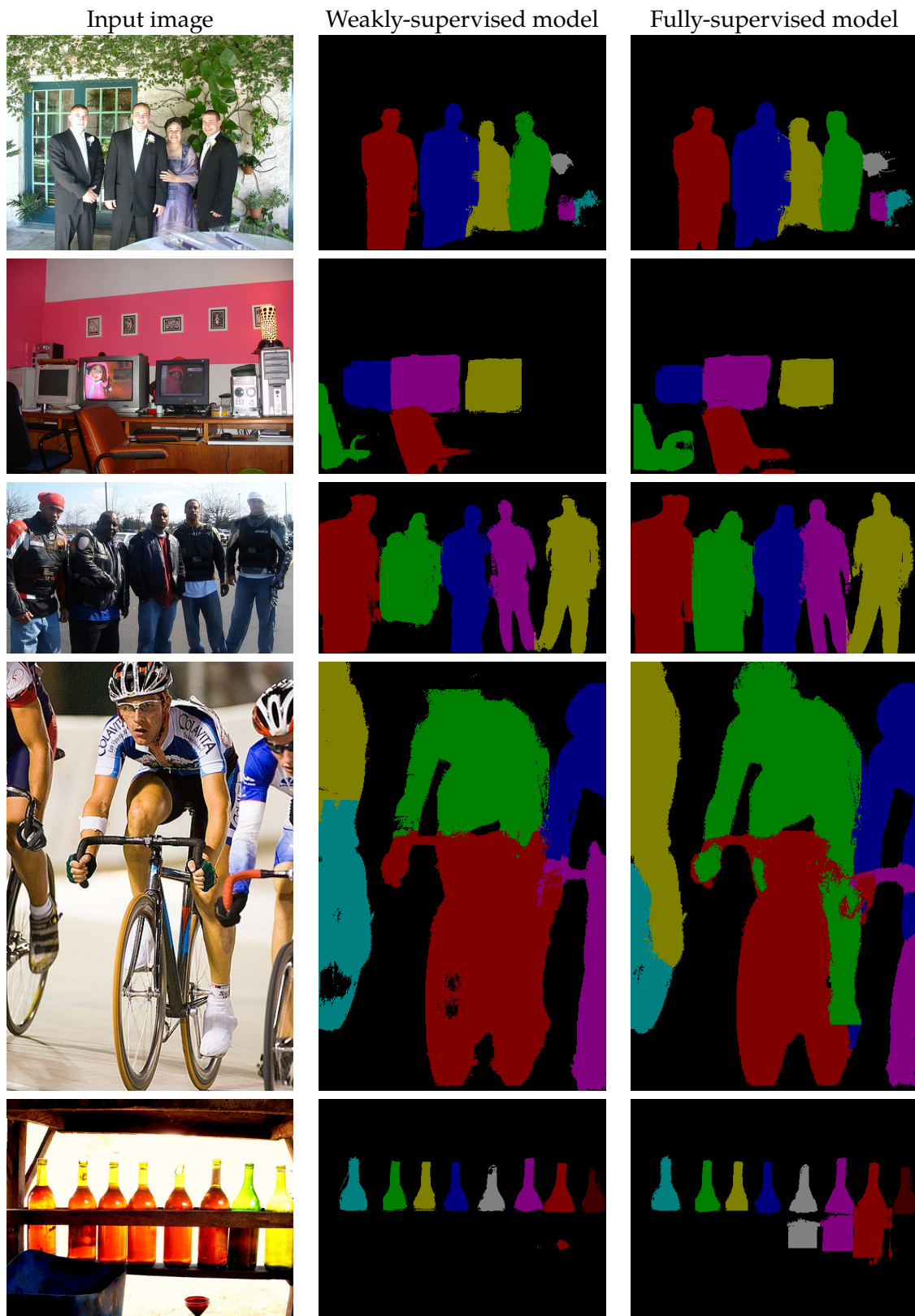
Figure 5.8 continued. The first and second rows show examples where the results of the two models are similar. In the third and fourth rows, the weakly-supervised model does not segment the “green person” as well as the fully-supervised model. In the last row, both weakly- and fully-supervised models have made an error in not completely segmenting each of the bottles.
