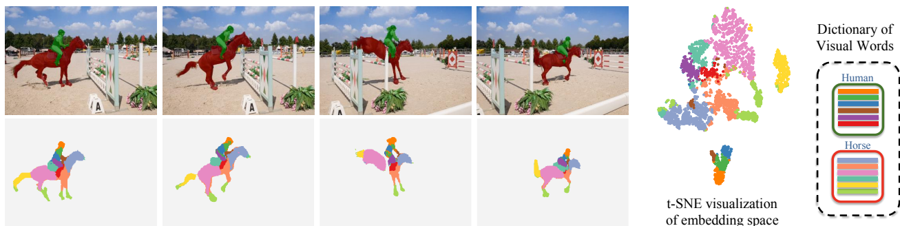
Figure 1: Video object segmentation using a dictionary of deep visual words. Our proposed method represents an object as a set of cluster centroids in a learned embedding space, or “visual words”, which correspond to object parts in image space (bottom row). This representation allows more robust and efficient matching as shown by our results (top row). The visual words are learned in an unsupervised manner, using meta-learning to ensure the training and inference procedures are identical. The t-SNE plot [29] on the right shows how different object parts cluster in different regions of the embedding space, and thus how our representation captures the multi-modal distribution of pixels constituting an object.
