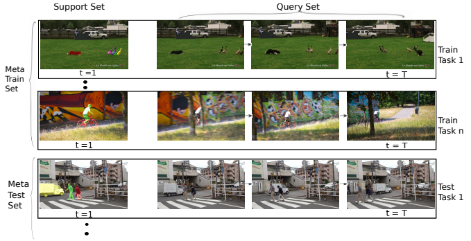
Figure 2: Formulation of video object segmentation as a meta learning problem. Each video presents a new task: Learn from the ground truth object masks on the first frame (support set), to segment them on the remaining frames in the video (query set).
