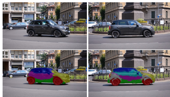
Figure 10: The effect of online adaptation on the representation of dynamic objects. As the object pose changes over time, newer visual words (denoted by gray and light-blue colors) are learned and added to the dictionary of visual words.
