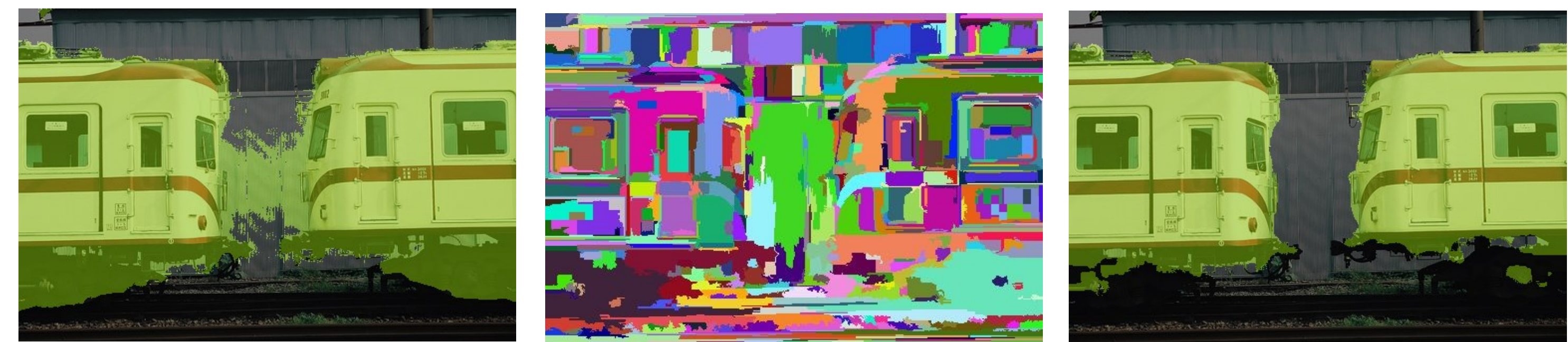
Figure 2: Output of system without superpixel potentials (left). Superpixels obtained from the method of [5]. Only one of the four "layers" is shown (middle). Note how the superpixel potentials get rid of spurious noise (right).
