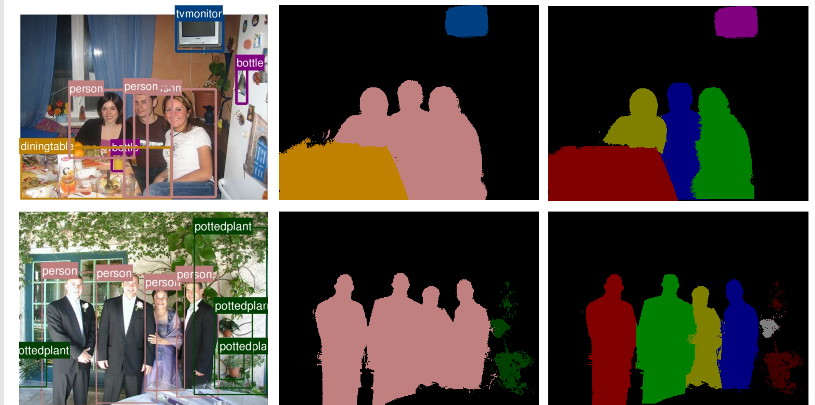
Figure 3: Left: Input image and object detections. Middle: Semantic Segmentation output. Right: Instance Segmentation output
