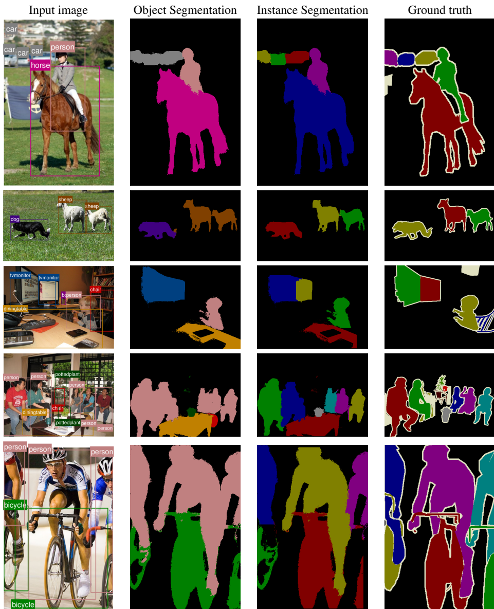
Figure 2: Some examples where our system has performed well. Detector outputs are overlaid on the input image. Top row: Our method is able to accurately segment the image, and distinguish the three cars in the background. Second row: Part of the dog’s tail, which was misclassified as “sheep” is not included in the instance segmentation of the dog. Third and fourth rows: The table (which is not annotated in either the semantic segmentation or instance segmentation ground truth), has been identified by our system. Fifth row: Both the category-level, and instance-level segmentations are quite accurate. Note how many false-positive detections have been correctly ignored by our system.
